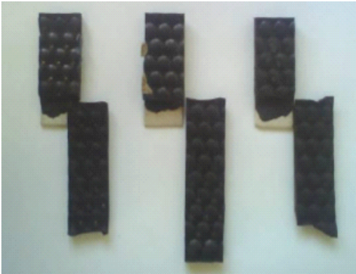
Figure 14: 90 Deg Peel test on UTM as per ASTM-D-429B.
