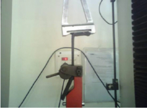
Figure 14: 90 Deg Peel test on UTM as per ASTM-D-429B.
