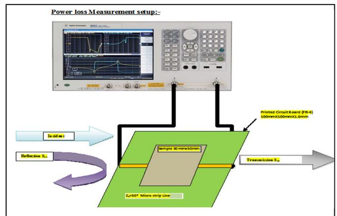
Fig.1. Microstrip Line Test setup for transmission attenuation Power loss measurement as per (IEC 62333)
