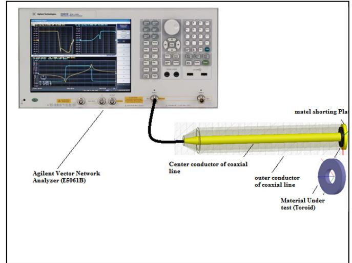
Fig.3. Air Coaxial Line Test setup for Reflection loss measurement as per IEEE-std-1128-1998
