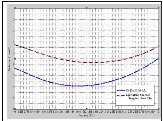
Fig.4. Comparative graph of Reflection loss between KV-SCA-SK-1 of SLTL and Equivalent Sheet of Supplier from USA
