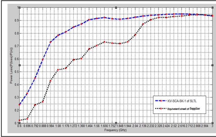
Fig.2. Comparative graph of Transmission attenuation Power loss between KV-SCA-SK-1 of SLTL and Equivalent Sheet of Supplier from USA
