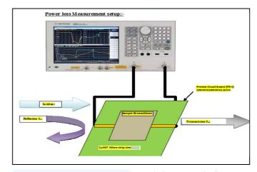
Fig.1. Microstrip Line Test setup for transmission attenuation Power loss measurement as per (IEC 62333)
