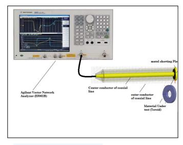
Fig.3. Air Coaxial Line Test setup for Reflection loss measurement as per IEEE-std-1128-1998  $\,$
