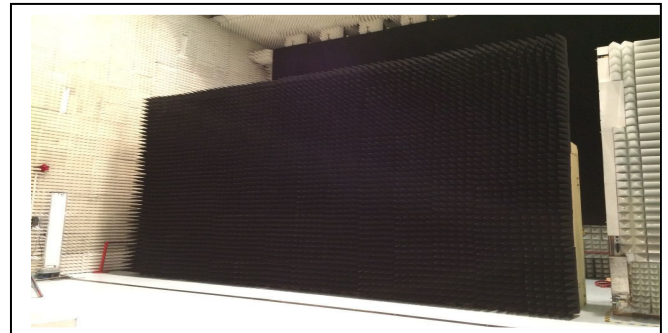
Fig.1. Clean Room Absorbers in European Space Agency (Thales Alenia Space)
